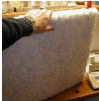
Insulation wool made from blade fibres via pyrolysis
