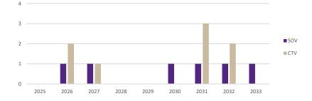
Figure 31 - Number of CTV or SOV required for Polish offshore wind farms, based on COD date
