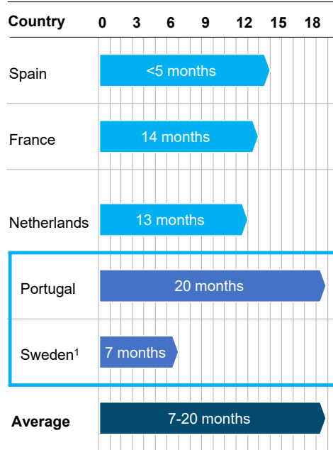
Time needed to install DC 150+kW chargers on highways, months
