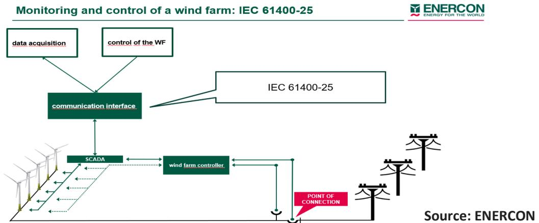
**Figure 8** Conceptual communication model of the IEC 61400-25 standard series<sup>11</sup>
