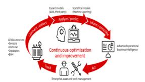
**Description:** The implemented Asset Performance Management (APM) solution provides actionable analysis results by collecting on-line operational information from the aggregator along with data from various sources - OT data from the historian, offline inspection data, nameplate data - and real-time analysis data through embedded or connected (via REST service) models, e.g. transformer expert models, kinetics models, machine learning models.
