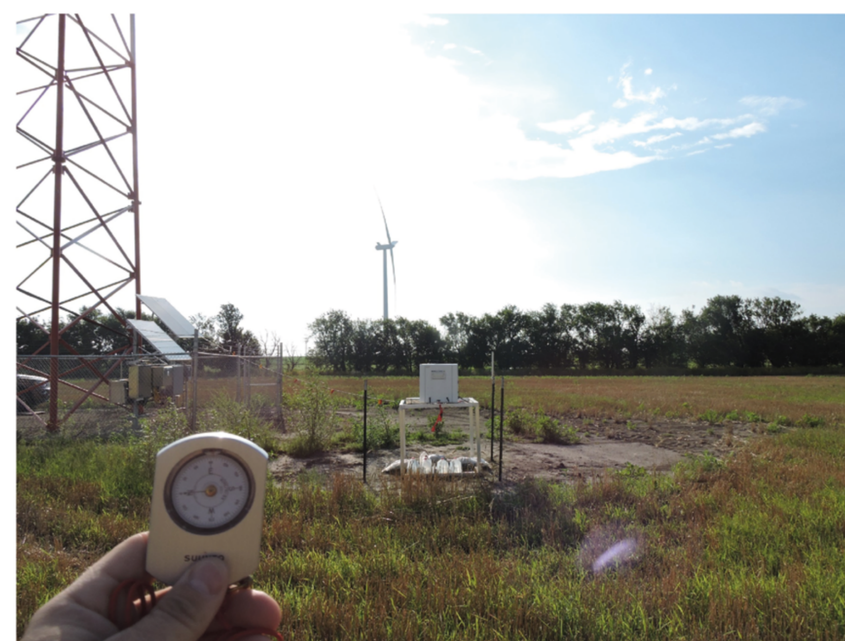
Figure 3: View of IEC compliant met tower and Windcube V2 profiling lidar
