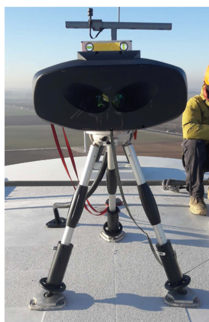
Wind Iris measuring at 80 to 400 m distance
