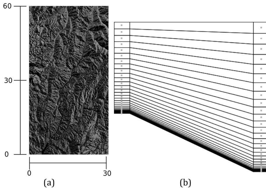
Figure 2. The x-y (a) mesh of the total region, and the vertical spacing of the mesh (b)
