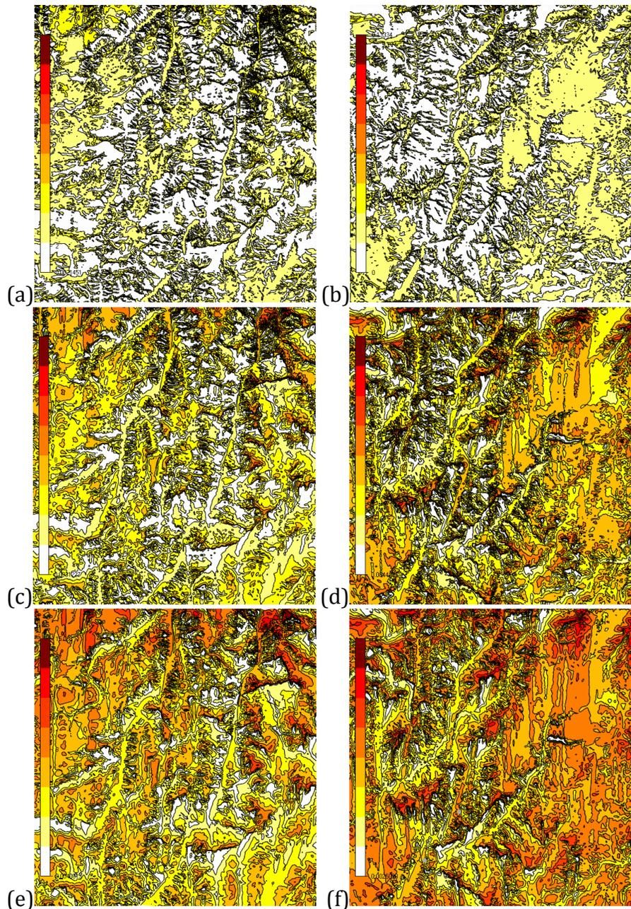
Figure 3. North (a,c,e) and South (b,d,f) sections showing wind speeds for one wind sector at 10, 50 and 100 meters above ground level – unscaled results.
