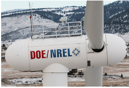
Figure 2: The 5-Beam Demonstrator installed on the nacelle of the CART2 at NREL. (Photo Credit: Lee Jay Fingersh, NREL 33621).
