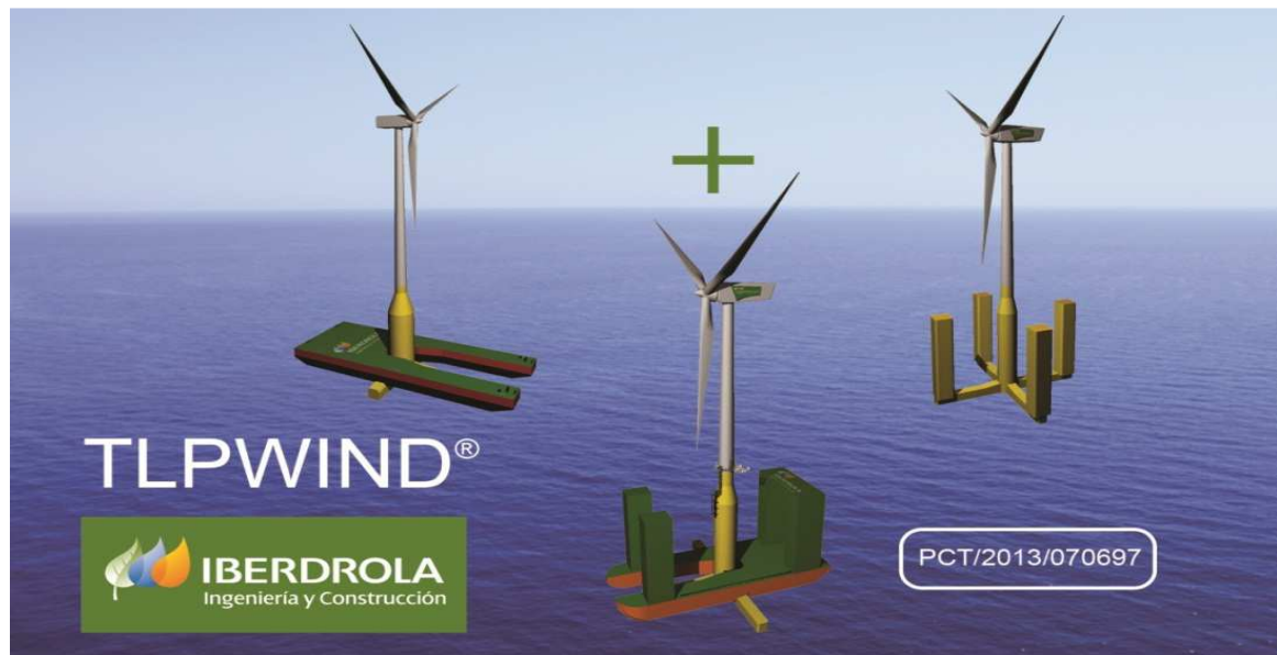
Figure 2-2 TLPWIND technology developed “ad-hoc” T&I solutions. U-shaped barge (left), re-usable floaters (right) and U-shaped semisubmersible barge (down) awarded with PCT/2013/070697
