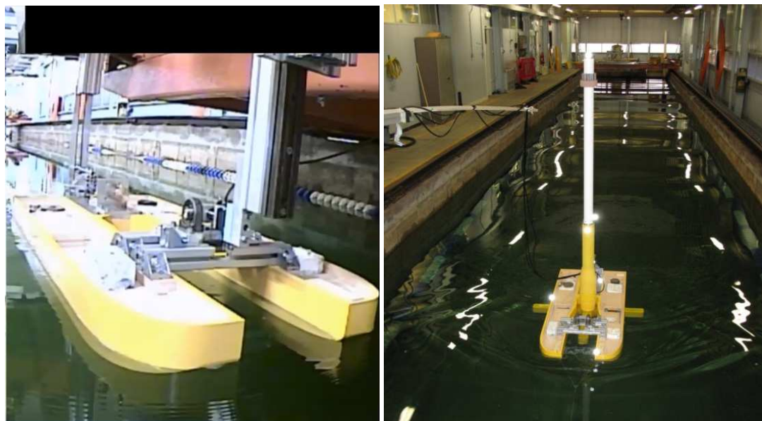
Figure 3-1 U-shaped SSB semi-captive towing methodology (left) and wired towing (right) extracted from videos recorded at Strathclyde's University basin facility
