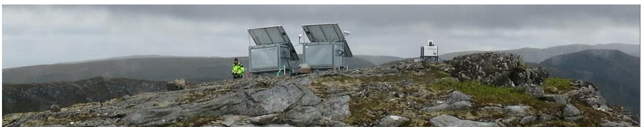
Figure 2 - Measurement setup with lidar system to the left and power supplies in the right of the picture.
