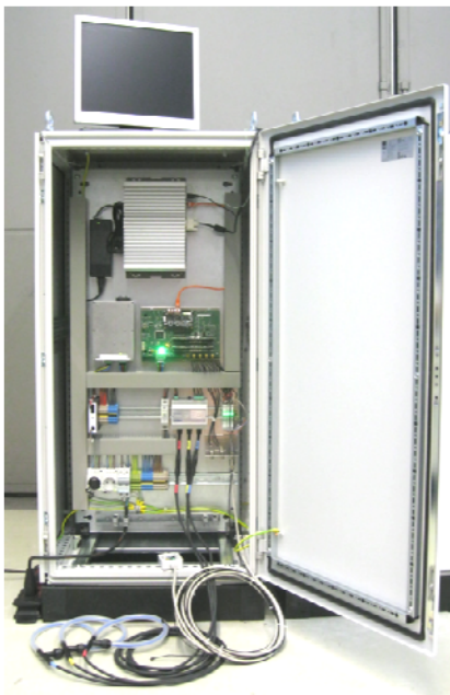
Fig. 1: Measurement Device, photograph and principle block diagram
