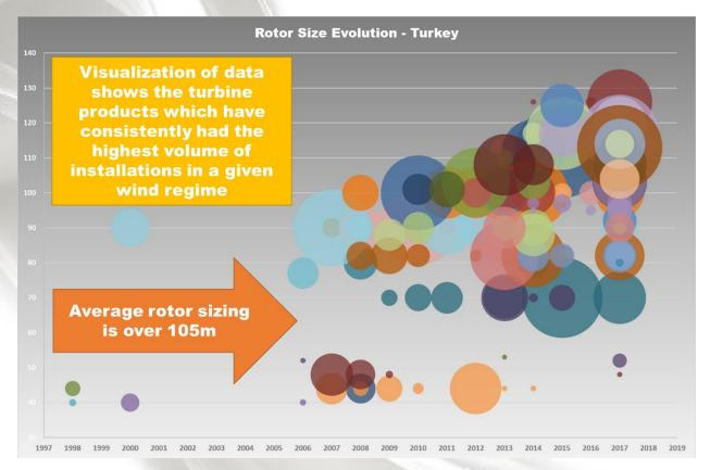
As before, a general trend in rotor sizing over time can be understood from data analysis. The chart indicates that average rotor sizing for the most competitive turbines in the market is over 105m.
