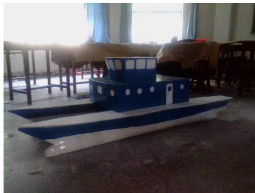
Fig.5 Ship model of the catamaran with big globular bow and stern
