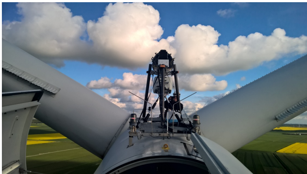
Figure 1 Picture of the Avent 5 beam demonstrator and the ZephiR Dual Mode lidars installed on the nacelle of a multi-megawatt wind turbine
