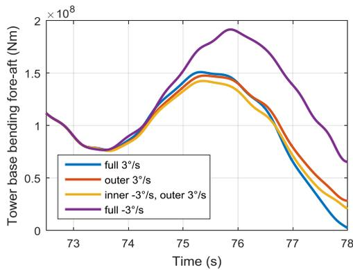
Figure 7: Tower base bending moment in fore-aft direction during an extreme event using different strategies of blade section movements.
