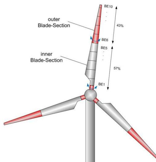
Figure 2: Division of blade sections on large-scale wind turbine for dual pitch.
