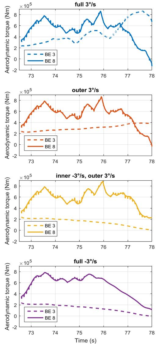
Figure 8: Aerodynamic torque blade element 3 (inner) and 8 (outer) during an extreme event using different strategies of blade section movements.
