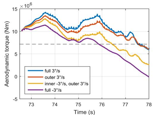
Figure 5: Aerodynamic torque during an extreme event using different strategies of blade section movements.
