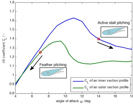
Figure 3: Lift coefficients for an outer and inner section profile during considered extreme event.
