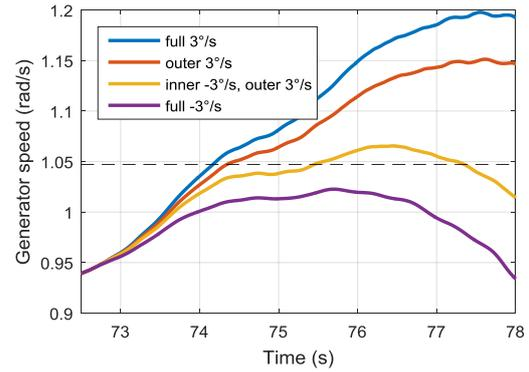
Figure 4: Generator speed during an extreme event using different strategies of blade section movements.
