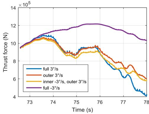
Figure 6: Aerodynamic thrust during an extreme event using different strategies of blade section movements.
