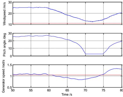
Figure 1: Changes in rotor-effective wind speed, pitch angle and generator speed during considered extreme event including rated values.
