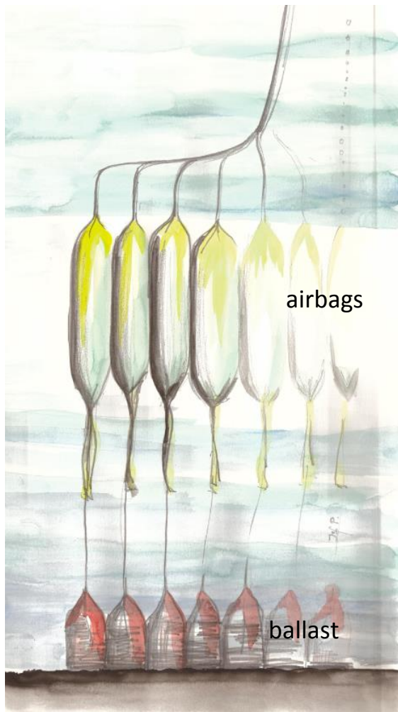
Figure 3 – concept : compressed air stored in airbags deep below the water surface
