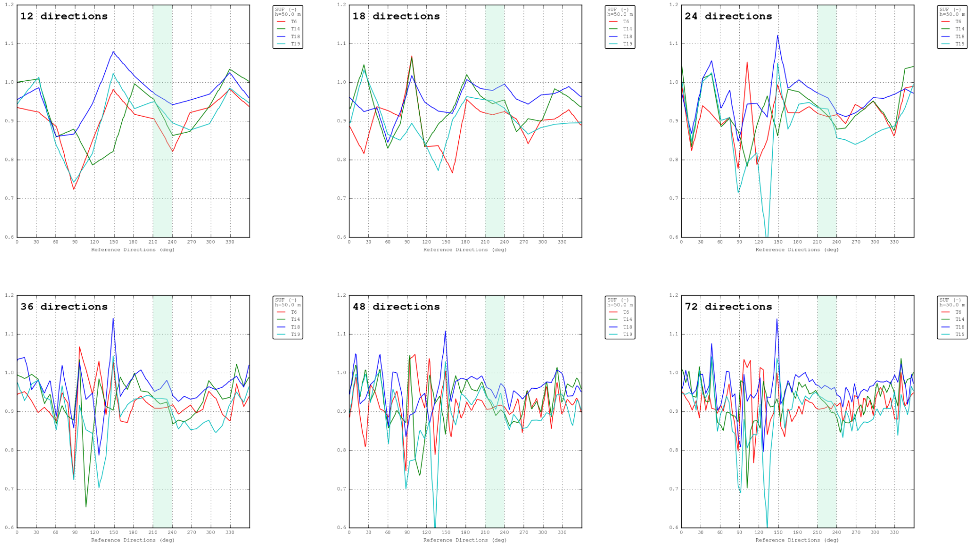
Figure 12: Speed-Up Results Interpolation against Wind Direction at Four Turbines Locations for Different Numbers of Computed Directions
