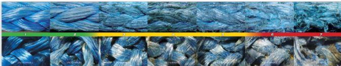
Figure.6. Visual comparator tool illustrating 7 levels of internal and external abrasion
