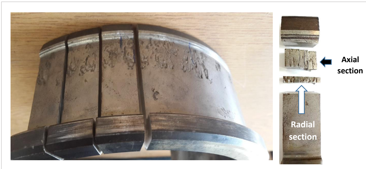
Figure 1: Main sections and subsections of the failed bearing
