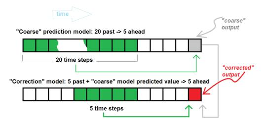
Figure 1. Double-module model: "coarse"-predicting module is using longer time-series of a single variable; the output from "coarse" module is utilized by "correcting" module along with shorter time-series of multiple variables.
