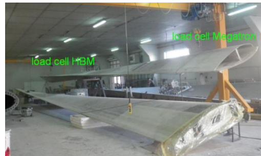
Figure 7: Photograph showing blade calibration
