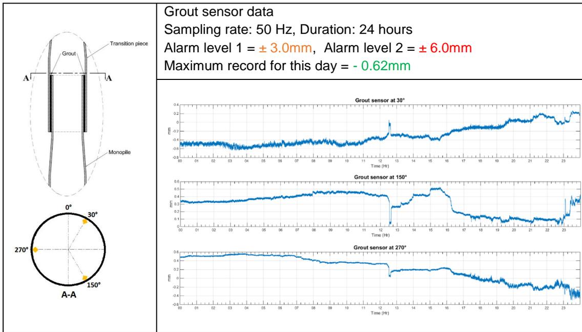
Figure 3: Stage I data visualization and alarm levels for continuous SHM
