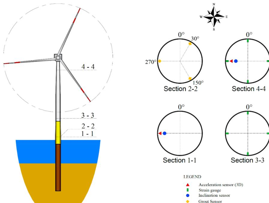
Figure 1: Typical vibration sensor positions for a global monitoring scheme
