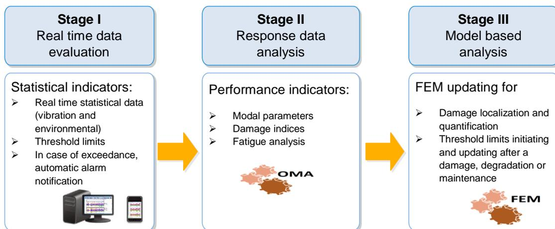
Figure 2: Three stage data evaluation strategy for continuous SHM data
