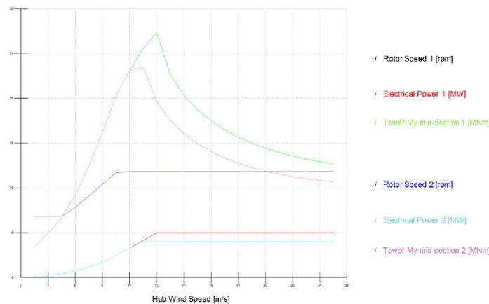
Figure 9. Principle Showing the Decoupling of Rotor Speed and Rotor Thrust
