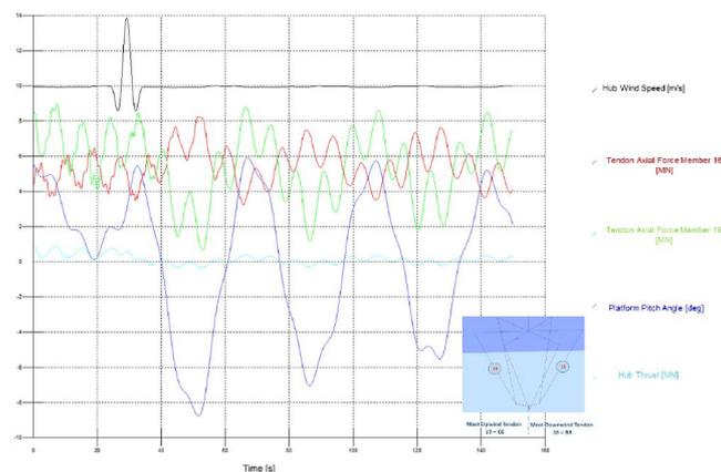
Figure 11. Axial Forces on Tendons Connecting Upper and Lower Tank
