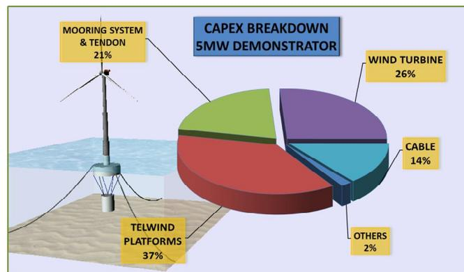
Figure 12. Capex Breakdown by main wind farm components
