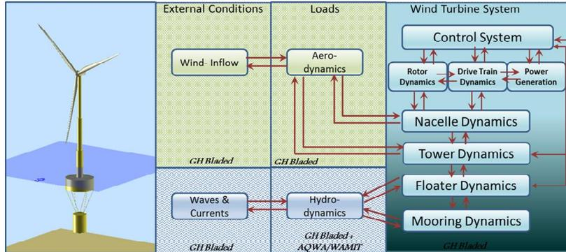
Figure 8. Interface Modules for Fully Coupled Aero-Hydro-Servo-Elastic Simulation
