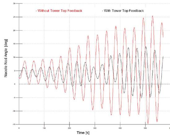
Figure 10. Platform Pitch Motion Damping with Tower Top Feedback at 20 m/s
