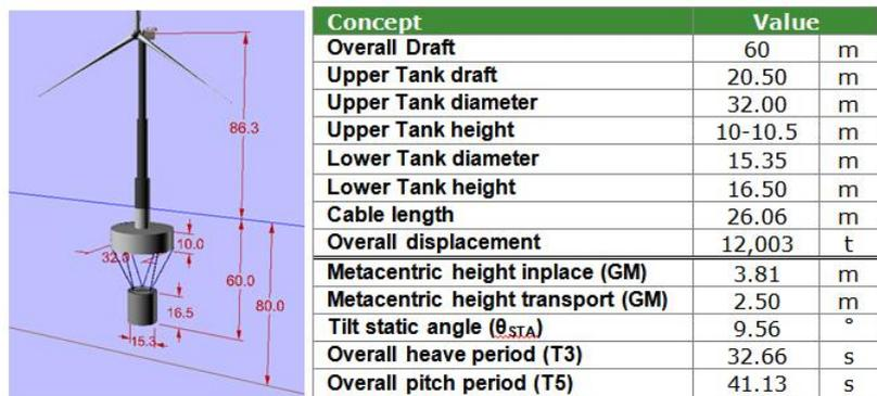
Figure 5. TELWIND preliminary design. Main characteristics.
