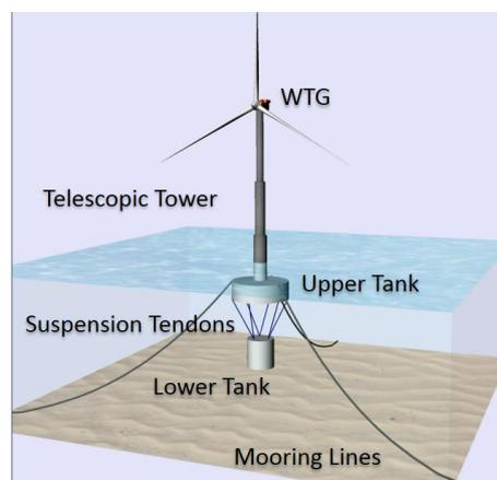
Figure 4. Showing the TELWIND main components
