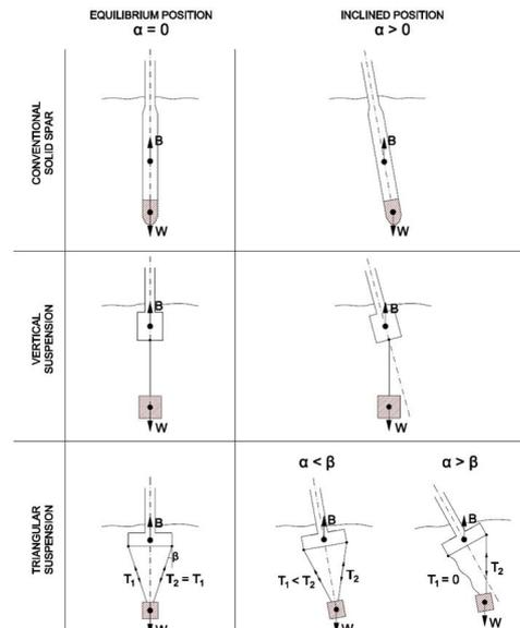
Figure 3. Conceptual fundamentals of the suspended ballast tank.
