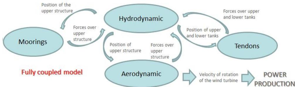
Figure 6 Fully coupled model scheme
