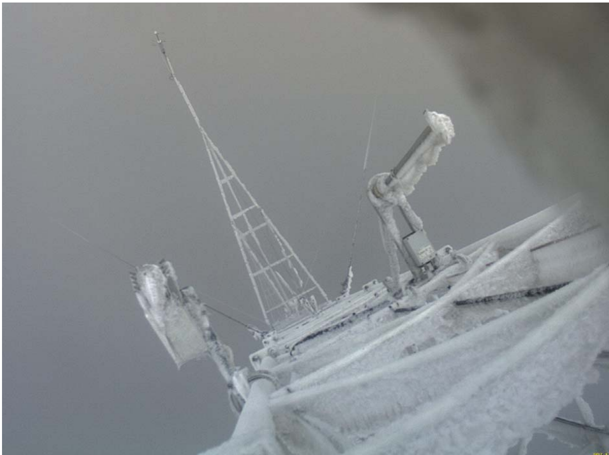
Fig.2: Top view of Iced met mast with ice sensors, camera and anemometry, middle icing intensity
