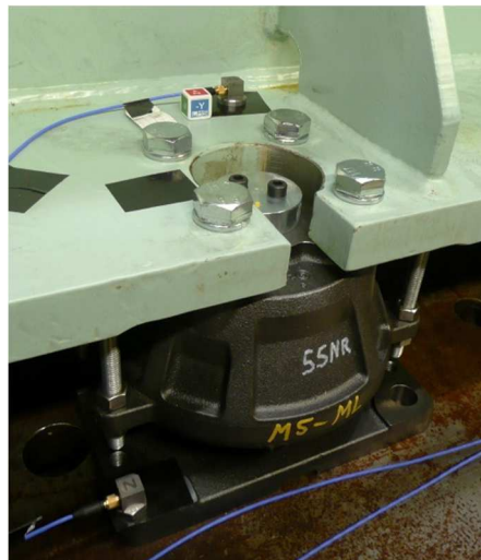
Figure 10: Left: Transmission loss of a single mass spring damper system excited by force (simulation). Right: on-site measurements of generator mountings.
