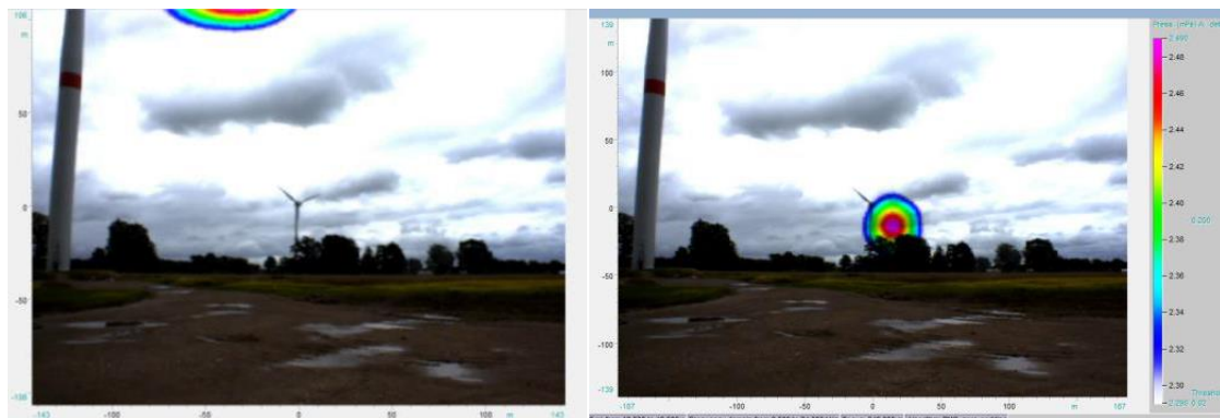
Figure 12: The wind turbine in the background (404 m apart) is targeted by removing the main blade noise component of the turbine in the foreground (149 m) using the acoustic eraser.
