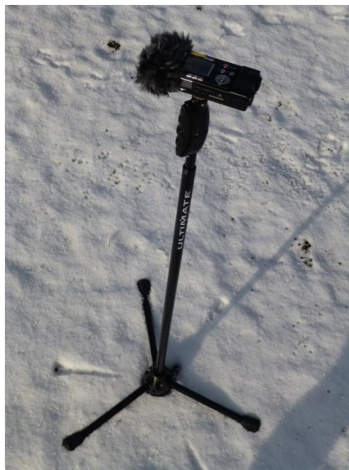
Figure 1: Used audio recorder system on a stand equipped with a wind shield
