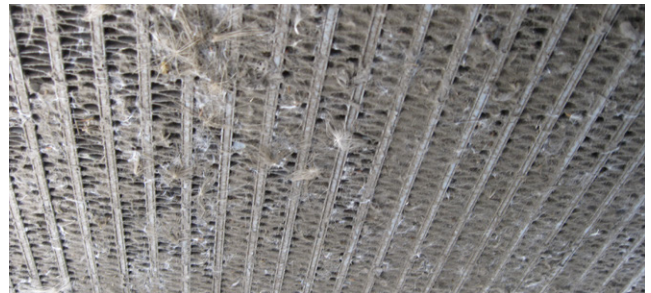
Debris from harvesting a nearby cotton field reduces the cooling effect. Diagnostic models can now detect this well in advance
