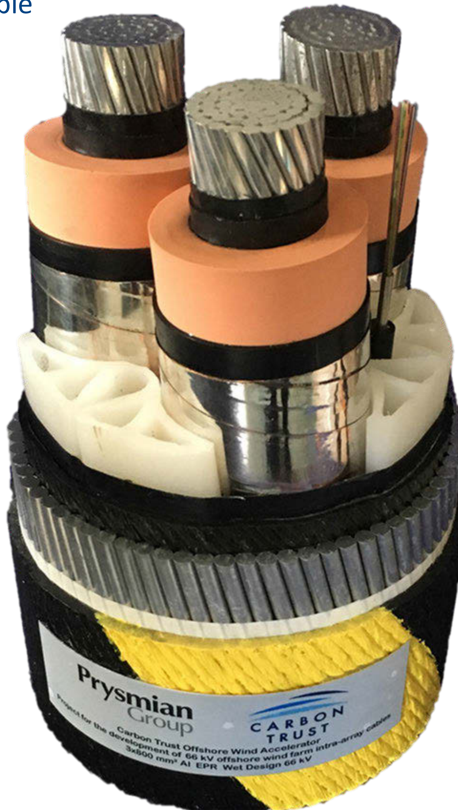
Example of 66 kV wet-design array cable with 800 mm 2 Al conductor and EPR insulation
