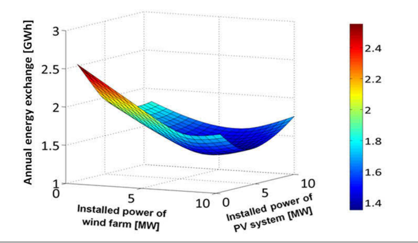
Energies exchanged between utility grid and the microgrid during each hour of the year, for the cases of optimization of RES installed capacity structure with and without DSM, are compared. The effect of introducing DSM is the decrease of the load on the feeder supplying the microgrid while the optimal capacity of the installed renewable sources increased from 10 MW to 12.5 MW.
