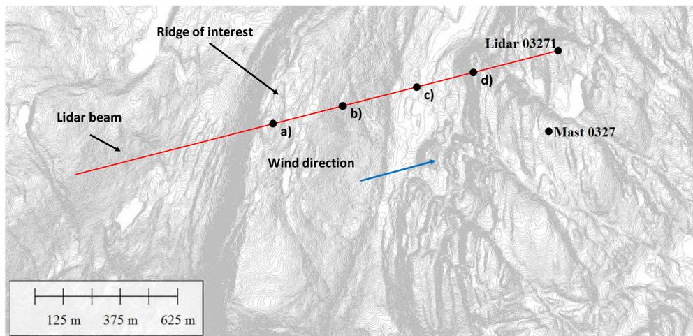
Figure 1 – Map describing the location of the lidar and measurement mast, as well as the ridge of interest to the study. The point locations a) – d) are used for further evaluations
