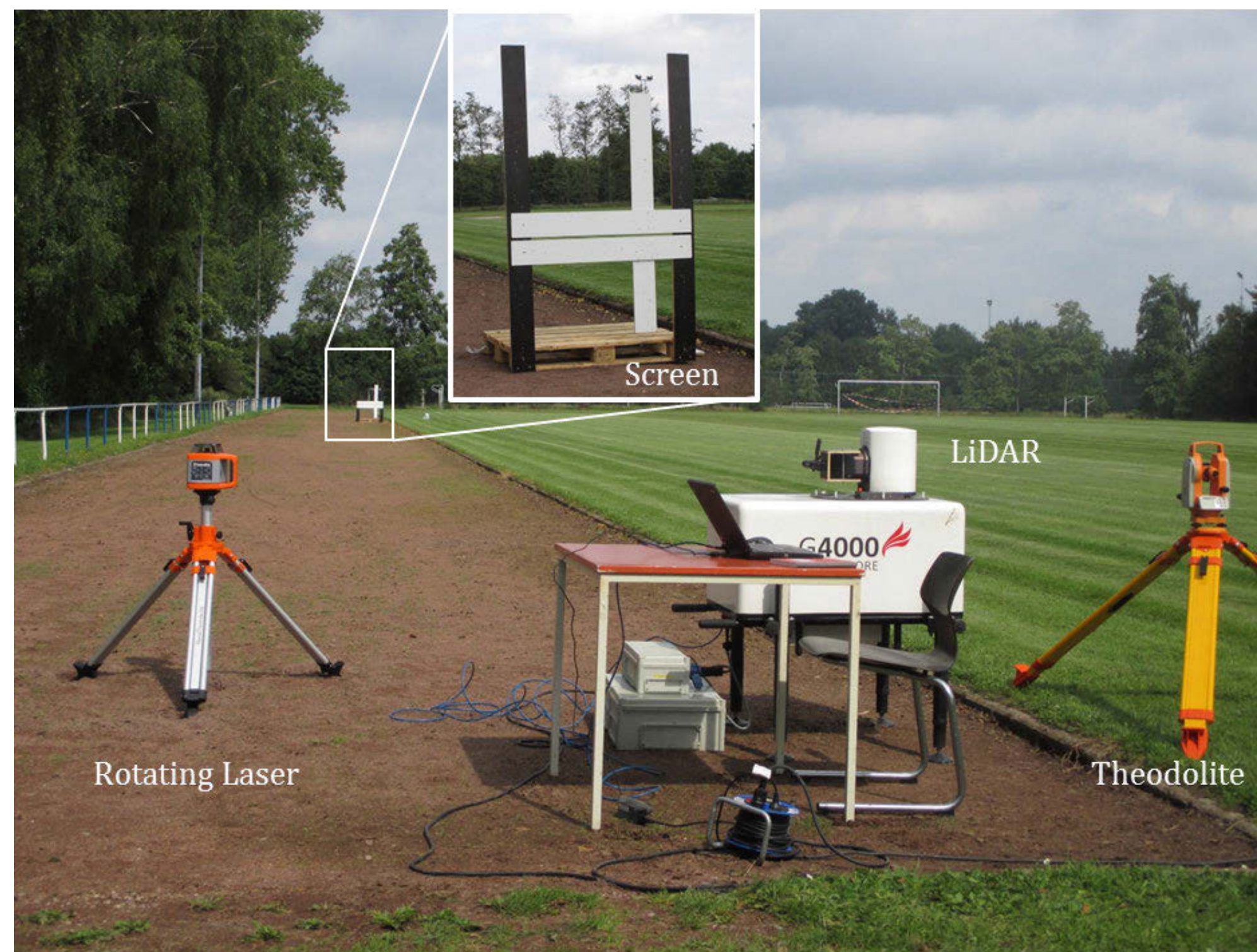
Figure 3: Picture of the experimental setup. The inset shows the screen. It is constructed to identify the location of the infrared laser beam of the LiDAR. The white panels are moved up to the point at which they just do not block the laser. The rotating laser defines a reference height across the measurement site
