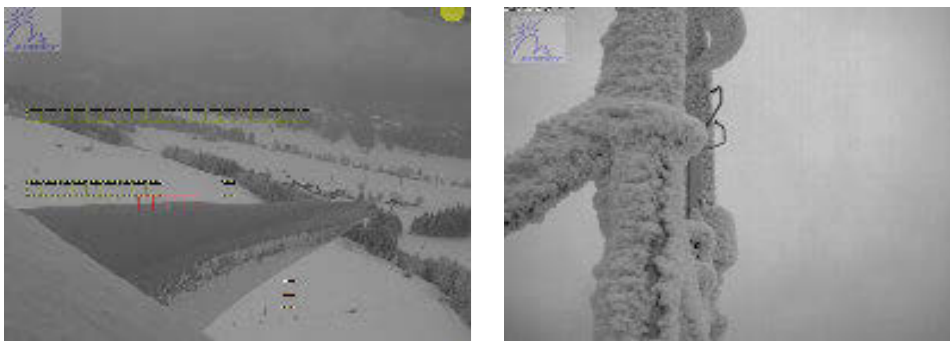
Figure 1: Webcams monitoring rotor blades (left) and anemometer on nacelle (right).
