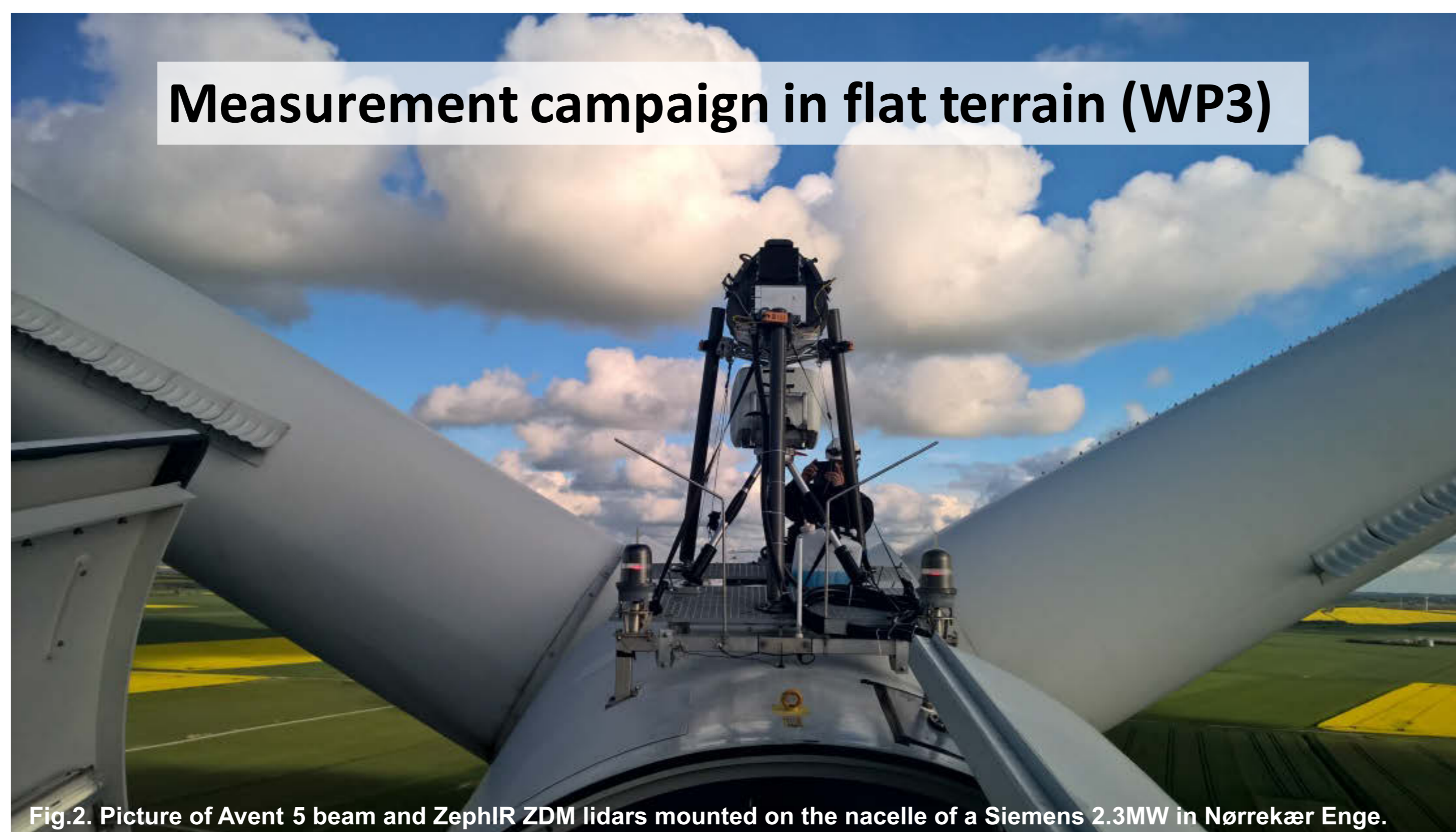
Fig.2. Picture of Avent 5 beam and ZephIR ZDM lidars mounted on the nacelle of a Siemens 2.3MW in Nørrekær Enge.
