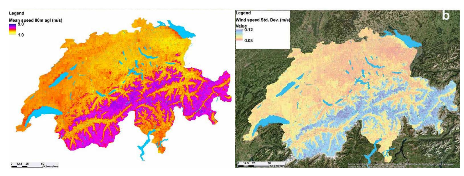
For each 1 km cell we are able to provide practitioners with the distribution of wind speed and direction, each with error bars to assess the long-term variability of the wind resource.
