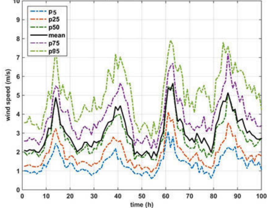
To demonstrate the effect of the wind variability on the electricity production we estimated the energy output on a single 2.3 MW turbine. From the image below is clear that even in hours of high average speed, its variability is an important factor to consider during planning.
