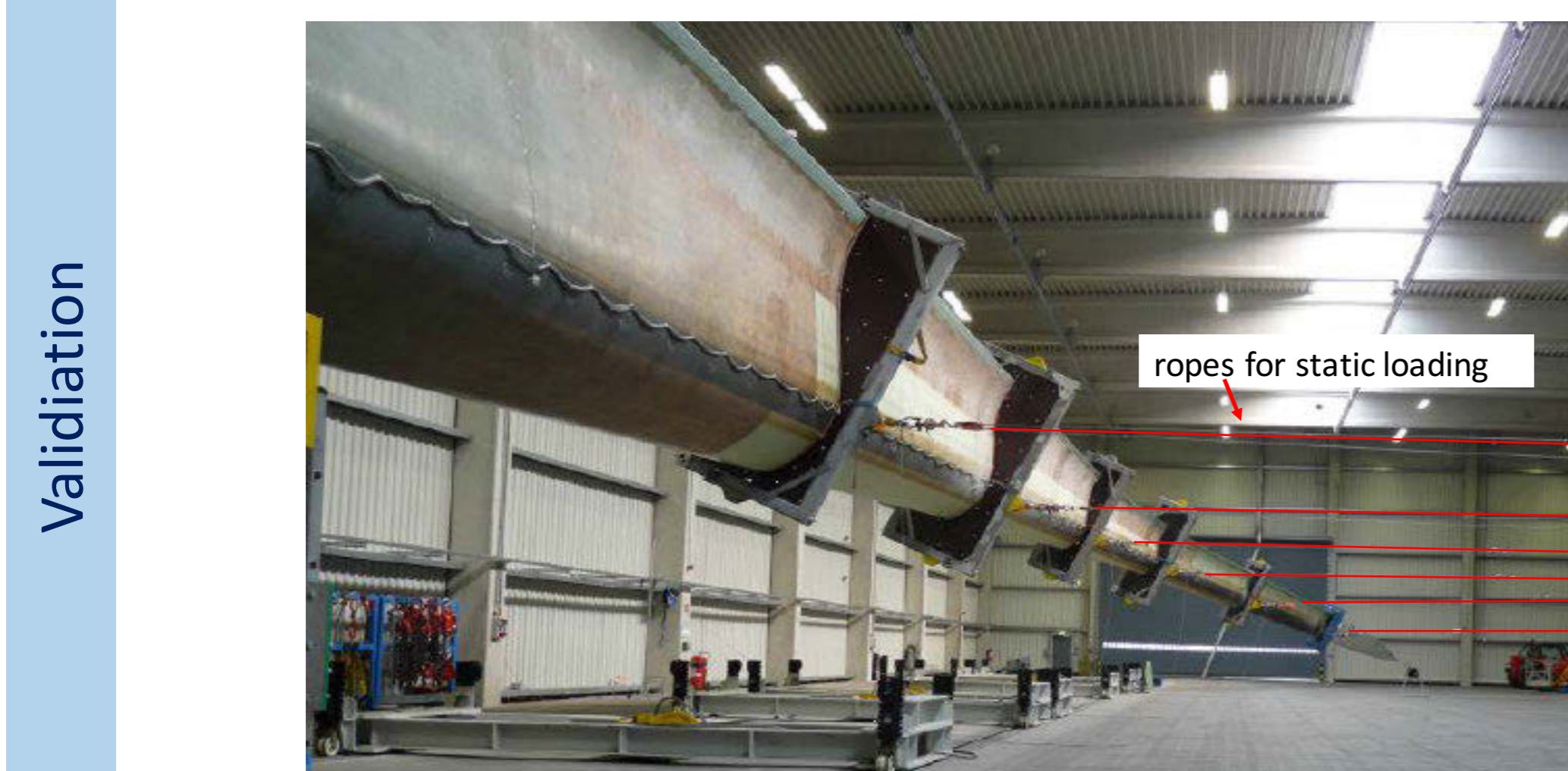
Static blade test at test rig, Nordex GmbH, Rostock
