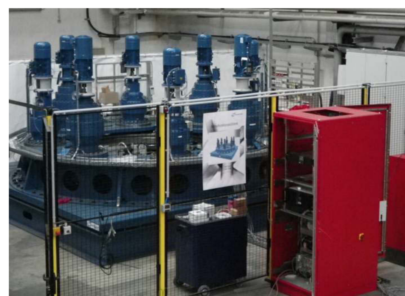
Yaw drives and load machines at test rig, Nordex GmbH, Rostock
