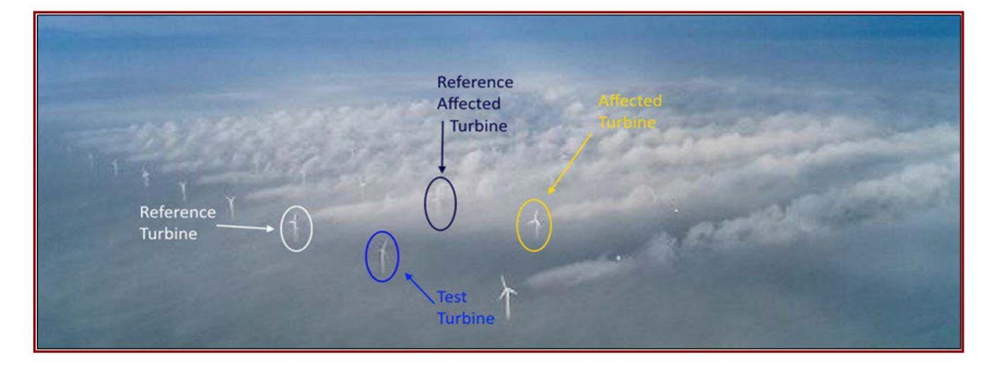
in normal operation: Available Power<sub>Test Turbine</sub> = Active Power<sub>Ref</sub> forence Turbine due to upstream curtailment: Active Power<sub>Affected Turbine</sub> > Active Power<sub>Ref</sub>. Affected Turbine</sub> what should be in normal operation: Available Power<sub>Affected Turbine</sub> = Active Power<sub>Ref</sub>. Affected Turbine</sub>
