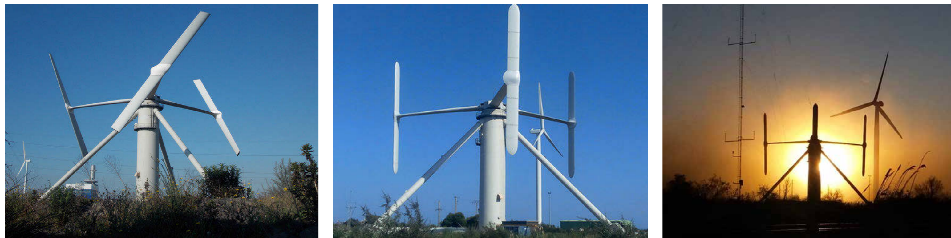
Fig.1: NENUPHAR's 600kW onshore large scale (height=42m,diameter = 50m) prototypes: 1H (left), 1HS (middle), view of the site showing 54m met-mast and 1HS prototype (right).
