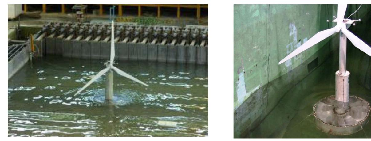
The design of TELWIND leads to a reduction of LCoE of offshore wind at deep water. The concept will provide important material savings of the floating structure, reduce installation costs by avoiding the need for offshore heavy lift equipment and keep the in-shore assembly works within limited drafts, heights and widths to profit from existing in-shore infrastructure.
