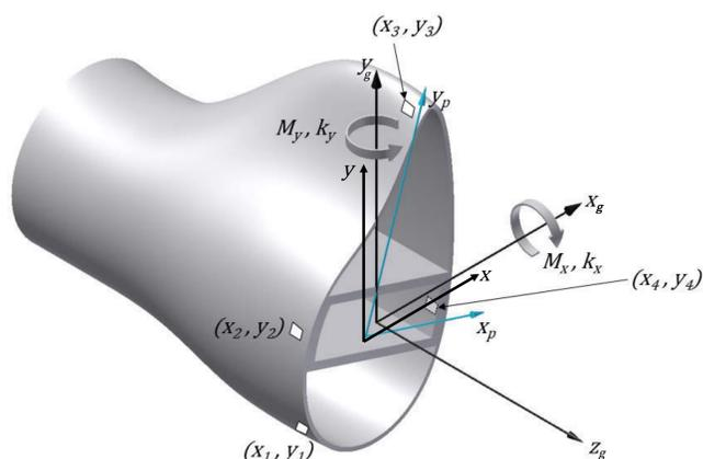
The axial strain at a given point on the blade can then be calculated from the standard equation for asymmetric bending of a beam:
