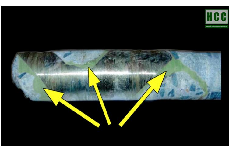
Also, it is noticed that the resin rises through the annular space between the ring and the pedestal, through the inner as well as outer area.
