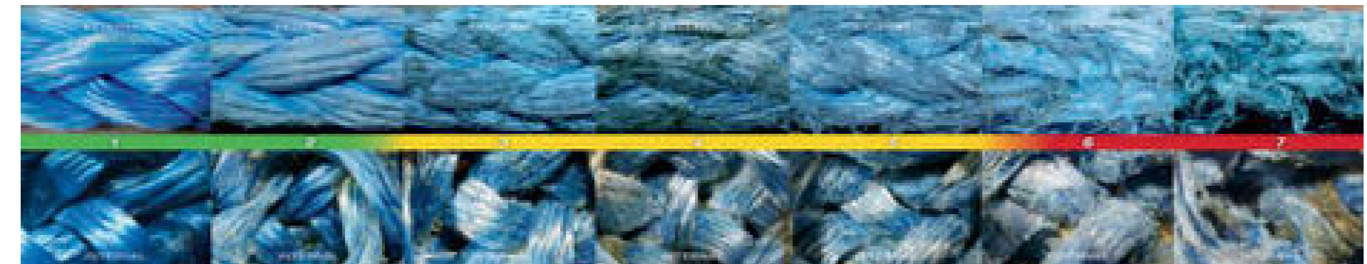
The visual comparator, above, allows comparison of both internal and external abrasion and indicates a general assessment of the rope's residual strength.
