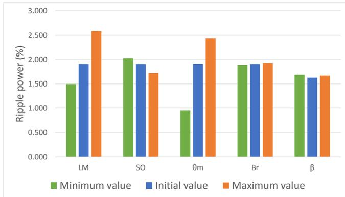
Fig. 8. Manufacturing tolerance influence in ripple power (%).
