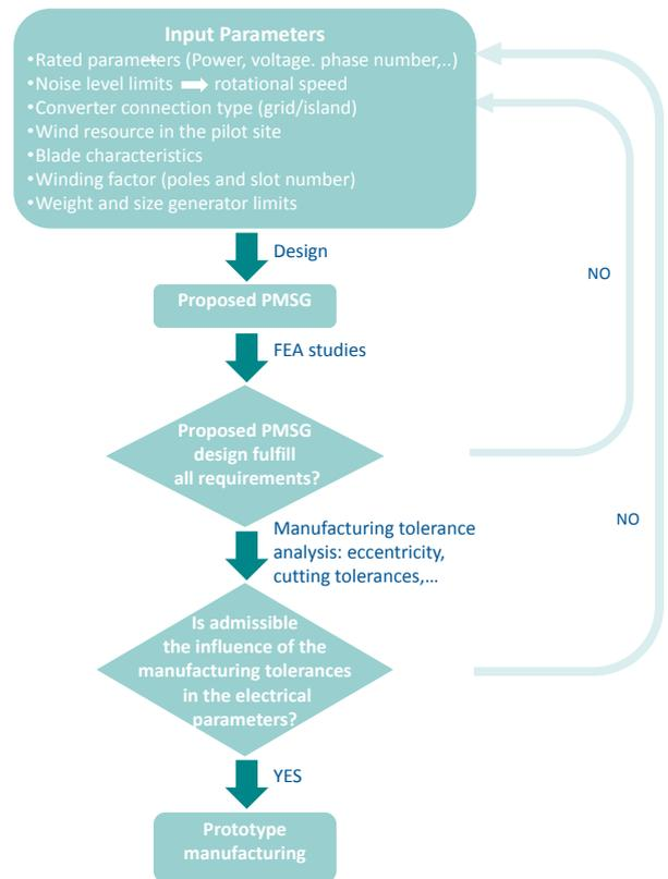
Fig. 1. Flowchart applied to the PMSG design.
