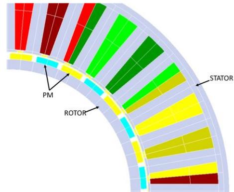
Fig. 4. 2D Finite element model PMSG.
