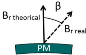
Fig. 2. Magnetic tolerances.
