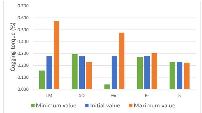
Fig. 6. Manufacturing tolerance influence in cogging torque (% Rated torque).
