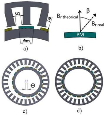
Fig. 5. Graphic representation of the tolerances under study. a) Dimensional tolerances; b) Magnetic tolerances; c) Static eccentricity; d) Dynamic eccentricity.
