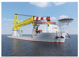
Les Alizés will mainly be used for the construction of offshore wind farms, but with her impressive crane she is also extremely suitable for decommissioning offshore oil and gas platforms.
