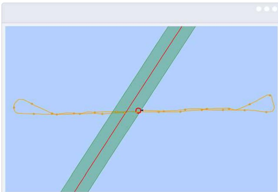
This image highlights how the service can be used to track vessel movements around a cable in its protection zone (cable: red, protection zone: green).
