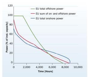
FIGURE 7: DURATION CURVES FOR THE 'WIND YEAR 2030'
