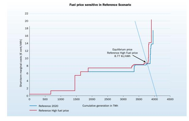
FIGURE 15: SENSITIVITY AND MERIT ORDER CURVE OF THE REFERENCE SCENARIO
