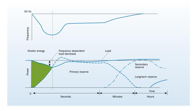
FIGURE 10: PRINCIPLE OF BALANCING IN THE POWER SYSTEM
