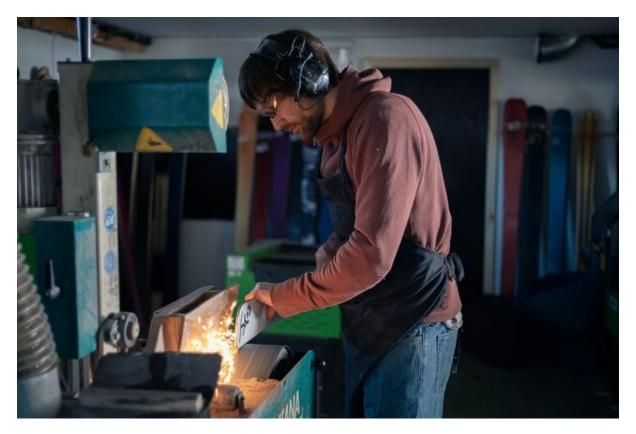
Endre Hals is the founder of Norwegian ski company EVI ski. Here he is demonstrating how the skis are manufactrured from decommissioned wind turbine blades.
