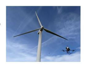
DOT's bespoke design allows it to manage the drone's cameras and automatically control how it takes photographs. It is simple to operate; the software can be linked to a tablet device to set up a turbine inspection and receive data. Crucially, the system reduces the need for skilled operators to undertake inspections, therefore lowering the chance for human error, due to its straightforward set-up process and sophisticated software.
