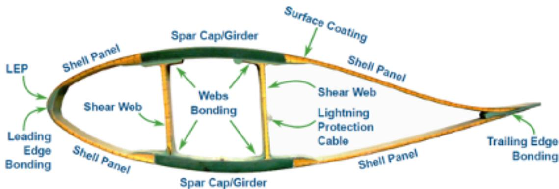
**Spar Caps/Girders:** Unidirectional (UD) Glass/Carbonfibre, supported by Epoxy, Polyester, Polyetherane or Vinylester matrix
